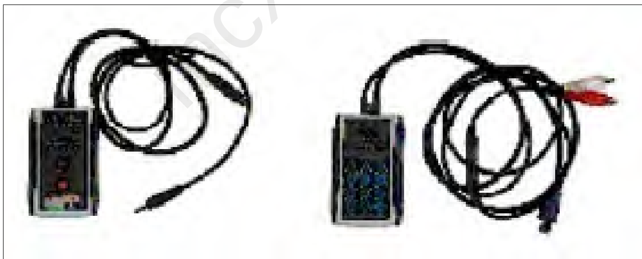
Fig 1: Identifying Original Multi-Media Interface Tester (105-00120-RCA) And New Multi-Media Interface Tester (105-00120-GEN2)
